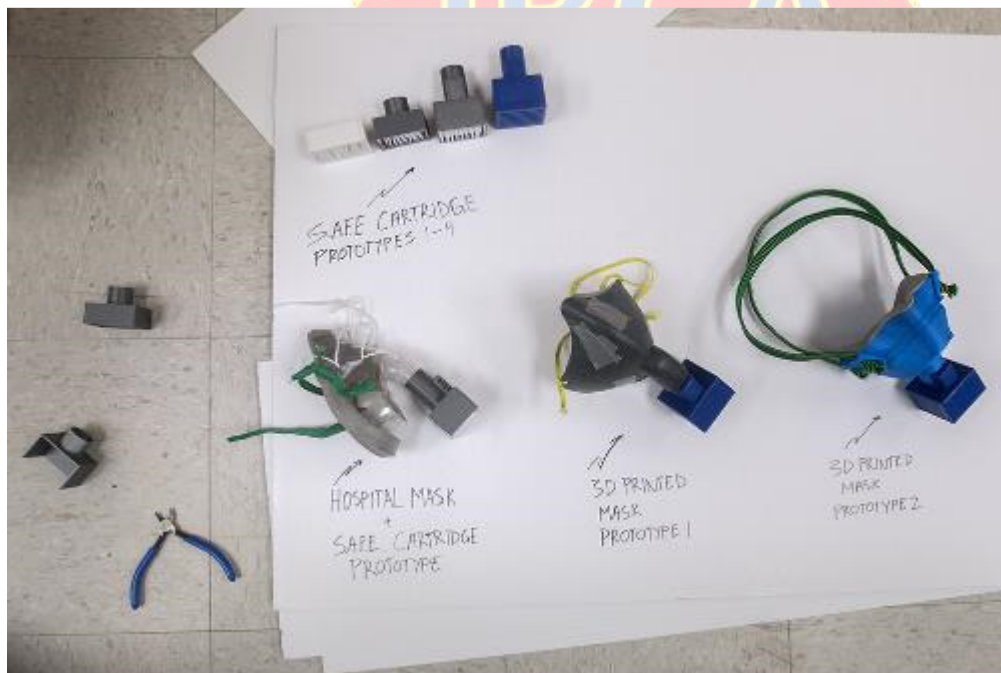
Image 1. MUSC design and prototype components of 3D-printed N95 respirator mask
