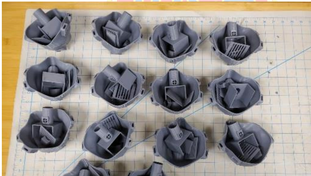
Image 3. 3D-printed N95 mask components ready for assembly
